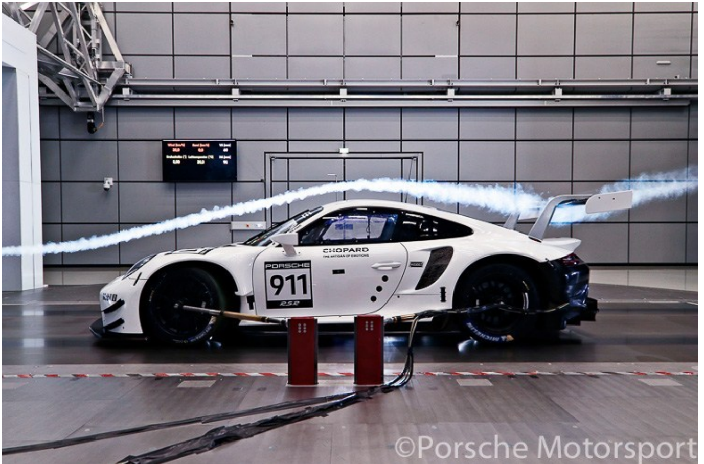
Development of the new Porsche 911 RSR (2019) in Porsche's wind tunnel at Weissach
